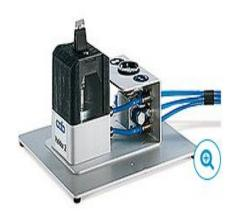
PCBs are separated carefully and quickly, off-cuts are removed precisely and smoothly. A two-part matrix enables the different blades to be assembled resp. exchanged easily.
