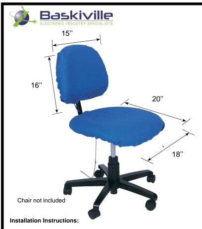
Attach top part of cover to chair back and bottom part of cover (with grounding chain attached) to chair seat. Make sure cover is fitted, centered, and secured to chair. Secure the ground chain to center post underneath chair with hook and loop and make sure ground chain makes contact with ESD floor. A minimum length of 6 inches of chain should make contact with the floor. For chairs with wheels make sure the chain is clear of the wheels so that it does not become entangled with the wheels.
