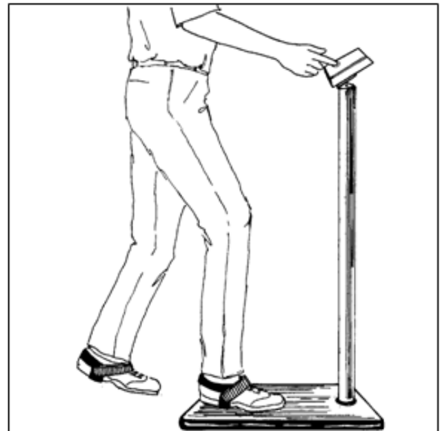
Figure 14. Performing a footwear test with the 19282 Combo Tester with Stand and Foot Plate
