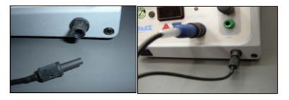
Connect foot pedal to foot pedal input on the back of your system.
