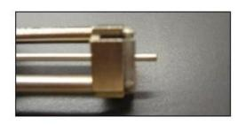
After partially inserting tip, align vacuum tupe with hole in tip.
