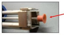
Insert suction cup onto end of vacuum tube.
